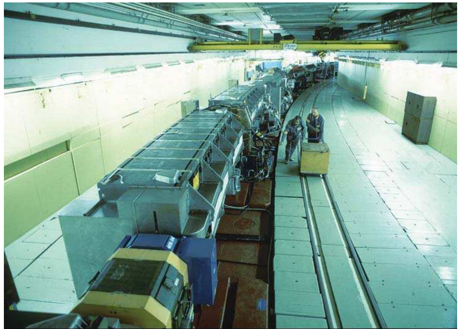
Figure 1 – CERN scientists accelerate and condition particles in the ring-shaped Proton Synchrotron.
